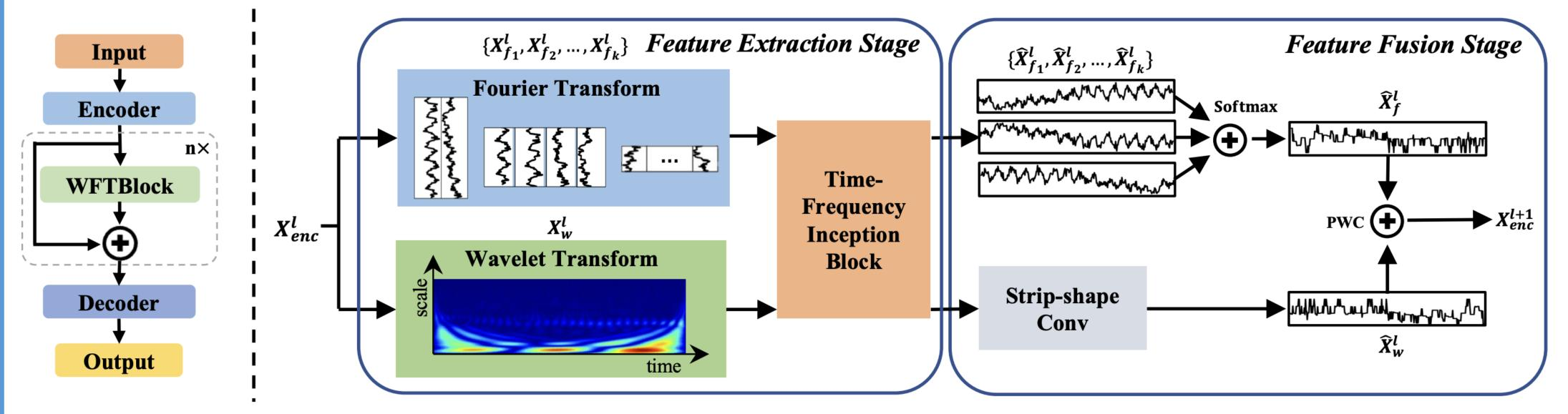
Overall architecture of WFTNet (left) and details of WFTBlock (right). The encoder and decoder manage input normalization, embedding, and output projection. WFTBlocks transform the 1D time series into 2D representations using FFT for global periodic patterns and CWT for local features.
